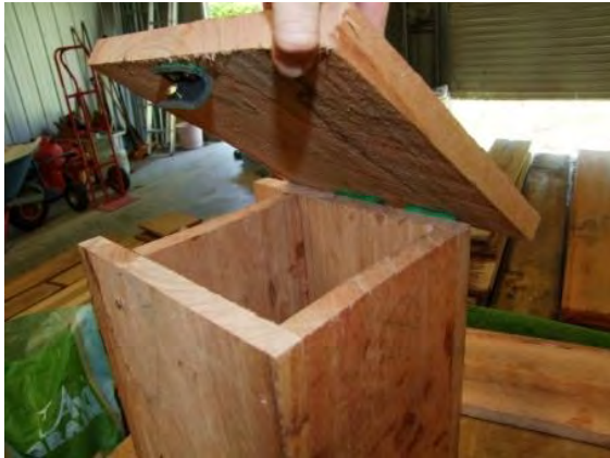
Figure 5. A durable hardwood box with 20-25mm thick timber
