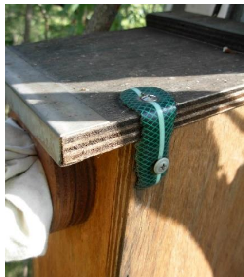
Figure 10. A strip of hose makes a good latch
